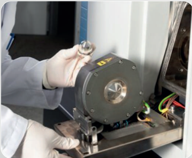
Figure 6. Easy Access Interface Door
