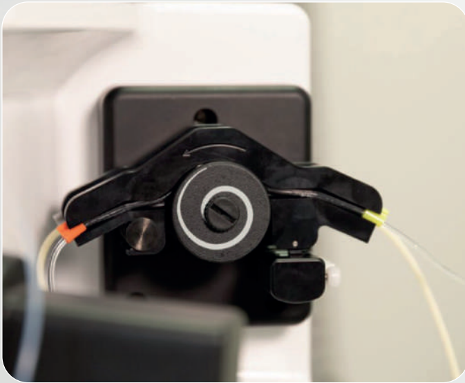
Figure 5. EasyClick Compact (ECC) Peristaltic Pump
